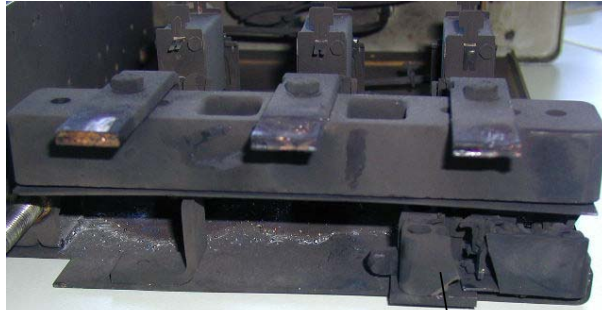
(2) Electrical contacts at rear of shutter
